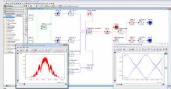
OptSim project layout of a DQPSK system. OptSim includes an advanced BER estimator specific for D(Q)PSK systems based on Karhunen-Loeve series expansion
